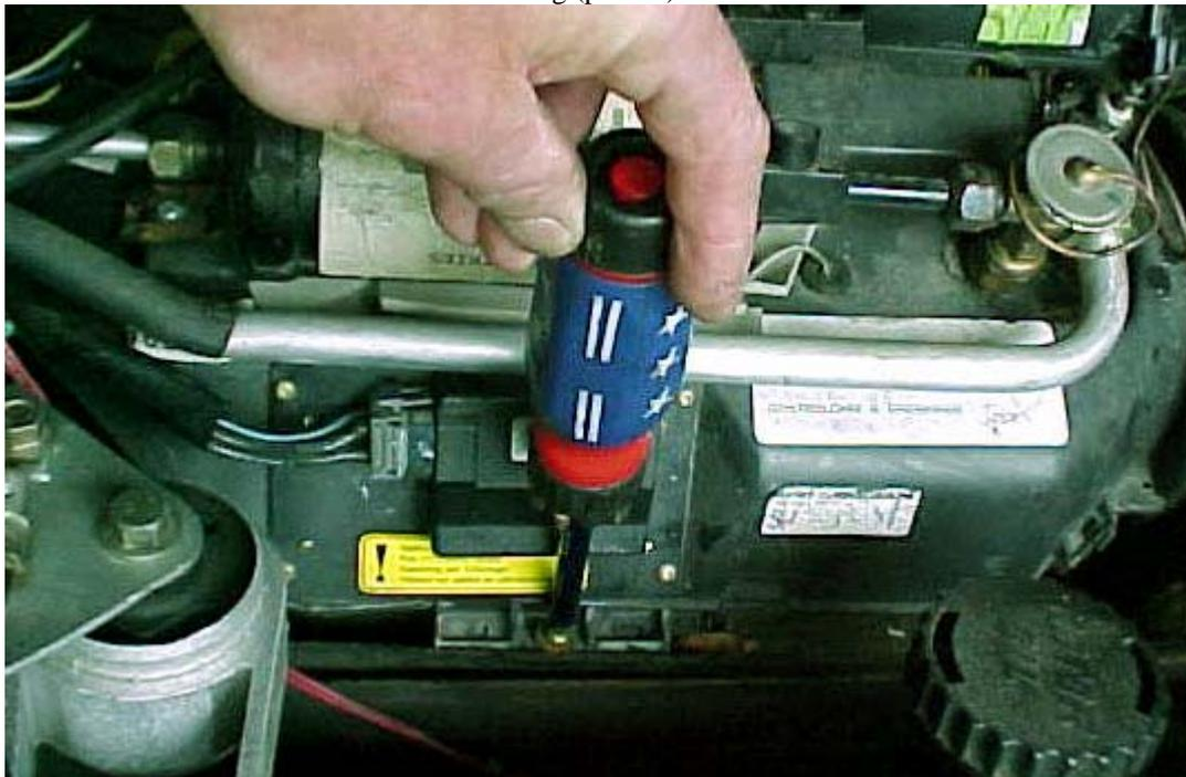
Remove the 10mm bolt that secures the power steering reservoir and the AC pipes.
