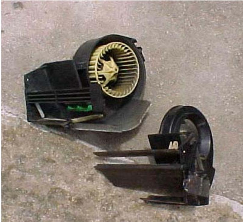
Remove the screw that holds the motor in (see previous pictures). I had to drive the motor out of the housing. First I reinserted the motor retaining screw and hammered on it until it bottomed. Then I used various long skinny screws/tools to drive it the rest of the way out. It was tight, and I pretty much destroyed the motor. Ridges in the housing make for a press fit for the motor. Some silicone spray on those ridges might make it go better. Picture
