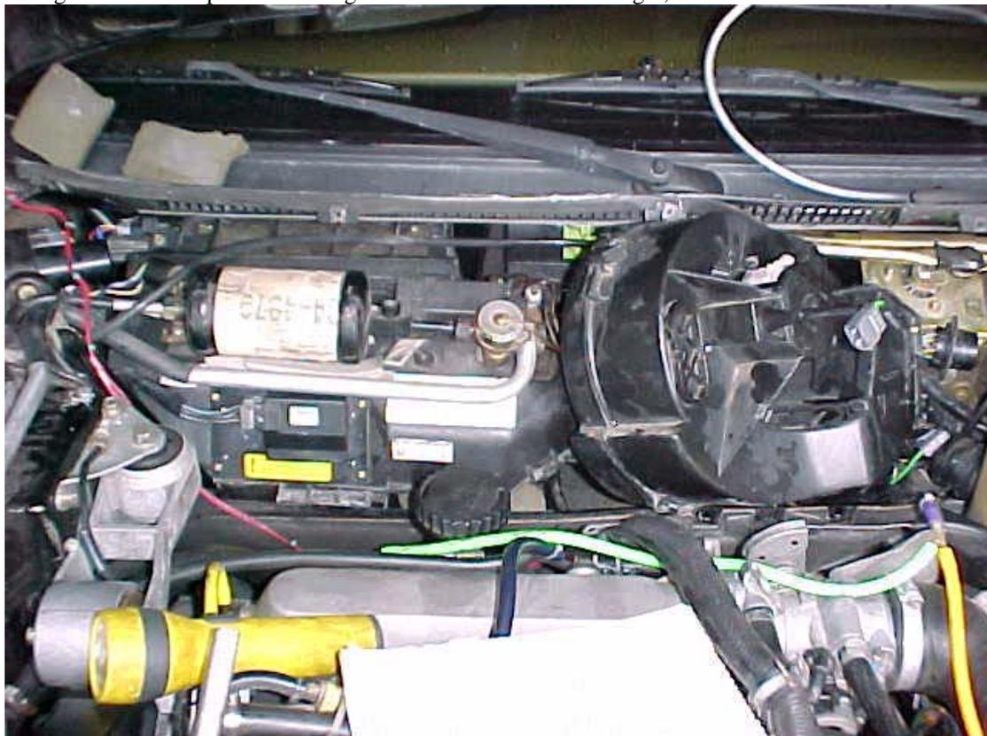
The evaporator has to be raised even higher to get the heater core out, and it gets really tight, but it CAN be done (picture).
