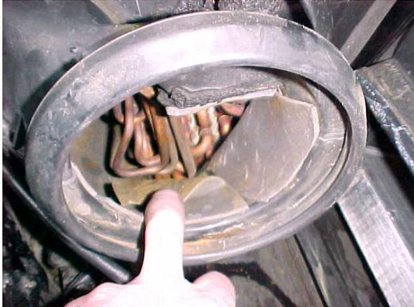
Loose insulation will end up in the fan, and cause failure of the fan controller. Use an aggressive rubber cement to glue any loose insulation back in place (some people say to remove the insulation). You can also remove the blower motor controller to gain access to the rest of it. Moisture tends to defeat the glue after a while. I found that the entire sheet covering the bottom of my evaporator housing was no longer glued down.
