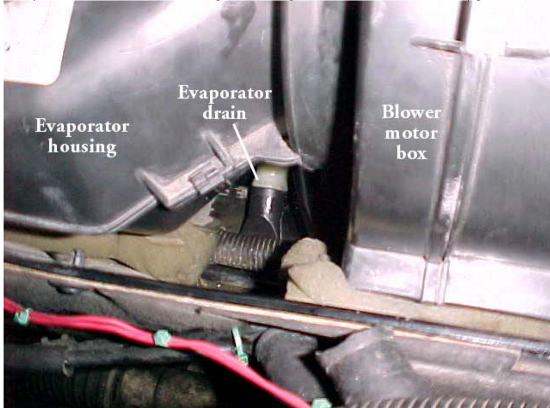
The evaporator drain goes down into a hole in the body pan. You can't quite see the hole here.
