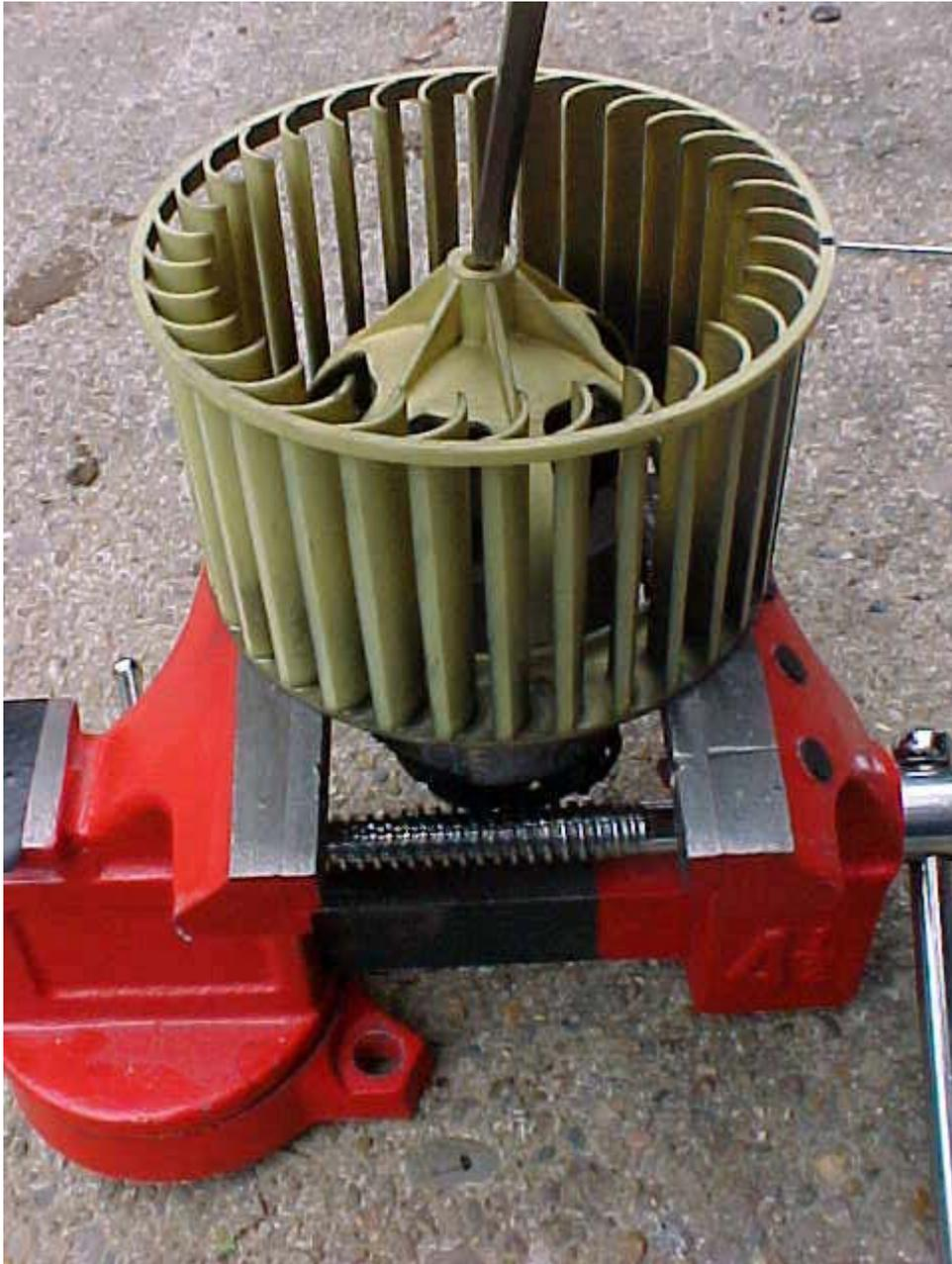
Rest the rear end of the shaft of the new motor on a solid surface, then gently tap the fan cage onto the shaft (picture).
