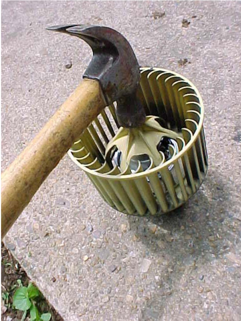
NOTE: It's important that the rear end of the SHAFT is supported when you drive the fan assembly onto the shaft. Grease the ridges in the housing and the new motor will slide right in. Don't forget to install the motor retaining screw. Reassemble the box halves, making sure that you get the flap linkage right (it can be tricky, but basically the flaps operate parallel to each other) Pictures.
