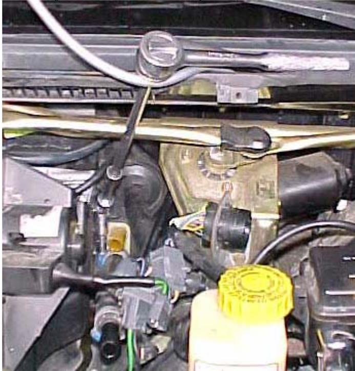
If you have quick disconnects rather than clamps, you have an original heater core and should consider changing it out for one that doesn't use quick disconnects.
