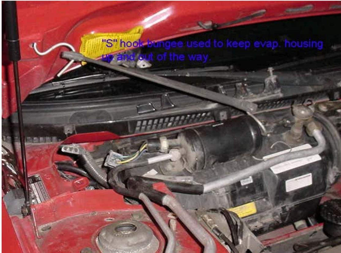
"S" hook bungee used to keep evap. housing up and out of the way.
