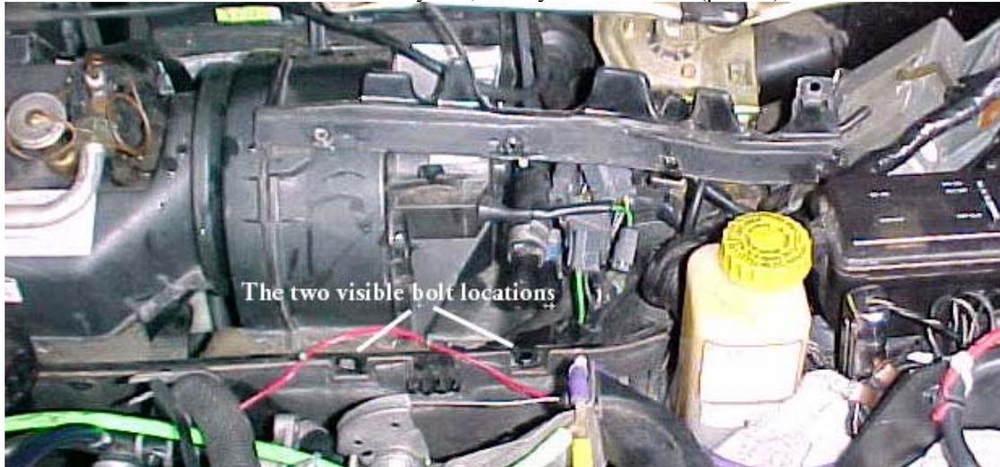
One is behind the ABS relay box (it is one son-of-a-bitch to get to); the other is directly beneath the wiring harness (picture).
