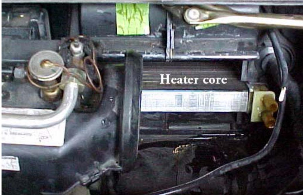
Separating the box halves - Remove the single (T20?) screw in the center. Remove the clips (four, if they're all there). Pry the front crossbar off. Separate the two halves of the box (pictures).
