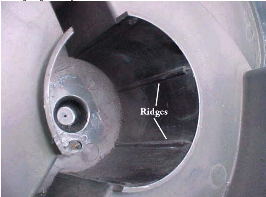
Replacing the motor - Support the back of the fan cage in a vise, then gently drive the motor shaft out (picture).
